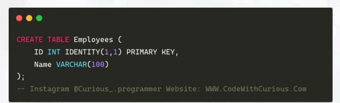
In this example, the ID column starts at 1 and increments by 1 for each new row inserted.
